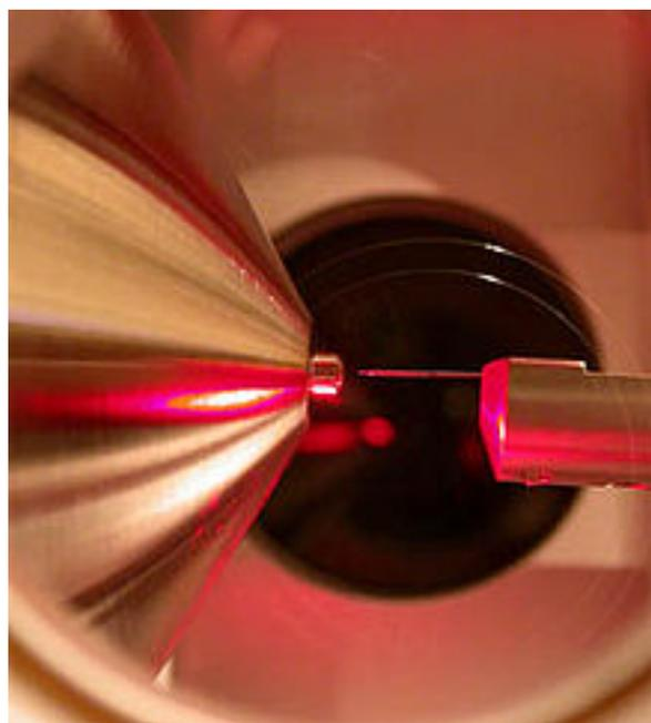
Picture of electrospray needle
